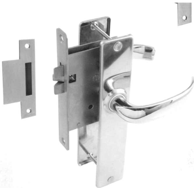
#18.2031 SET Passage door lock 50 mm backset. Face plate: 144 x 22 x 2 mm; Lock case: 95 high x 75 wide x 13 mm thick. Escutcheon plate: 196 x 38 mm, Lever 110mm long overall. Marine grade; stainless steel and brass chrome plated parts.
